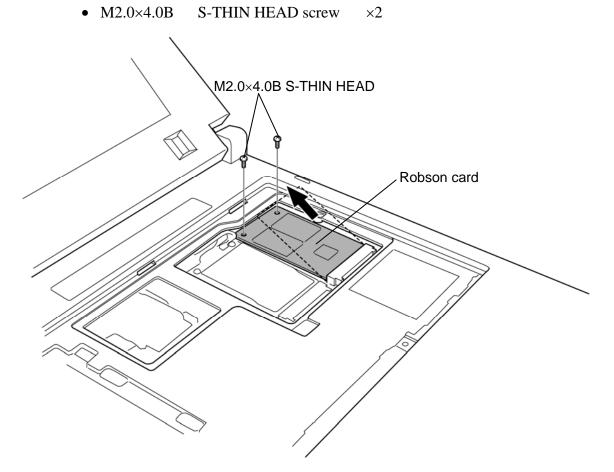
Figure 4-21 Removing the Robson card
